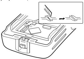
**NOTE:** Be sure to re-solder the disconnected points at left, otherwise no TX modulation or AF output is available when you remove the scrambler units.
