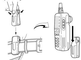
④ Once the transceiver is locked in place, it swivels as illustrated below.
