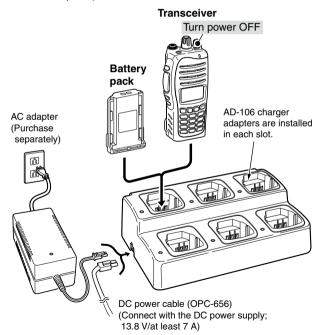
**IMPORTANT:** Ensure the sides of the battery pack are correctly aligned with the charger groves.
